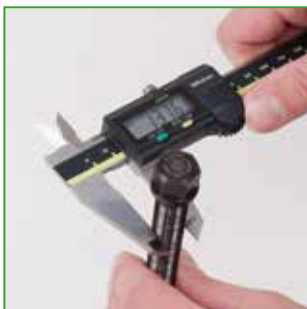
a Measure the spindle diameter.
